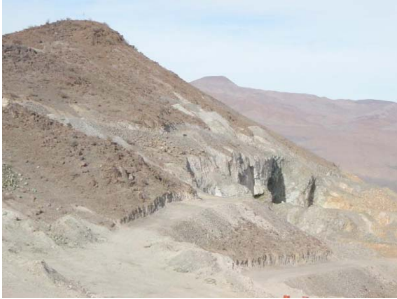
Figure 6. View looking southwest at Manto Pit. Mineralized zone dips to the southeast, to the left in the photo.
